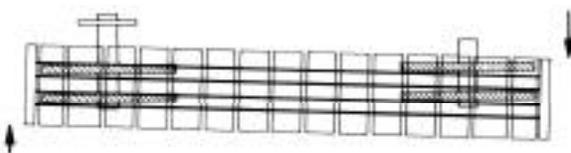
Rotate Track forward and work the Track inward until the Track's Inner & Outer Chains align and engage the teeth of their mating Inner & Outer Sprockets on the Front Idler.
